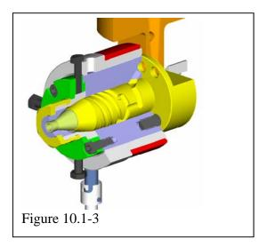
strength, for no weld lines will exist in the product. The best aesthetics of the extruded product are also produced with this method.
