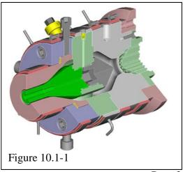
An in-line, center-fed die is the preferred method for polymer processing, as this design will generally provide the least damaging path for the melt flow. Spider and spiral type in-line heads are still the mainstay of tube and pipe extrusion production. The strainer-basket designs are being gradually replaced by the spiral distributor heads. This exchange is primarily due to lower manufacturing costs and improved product physical properties with the spiral heads.
