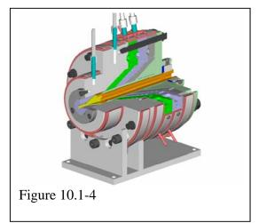
For example, in a three-layer cylindrical spiral forming head, the volume, and therefore the residence time increase between the innermost and middle cylinders can be 50%. The increase from the middle cylinder to the outer cylinder can be 35%. From the inner to the outer cylinders can be an increase in volume of 100%.
