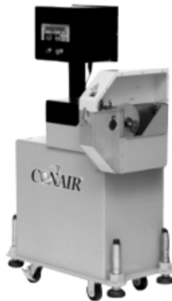
Figure 11. Fly-knife cutter. (Courtesy of Conair)
