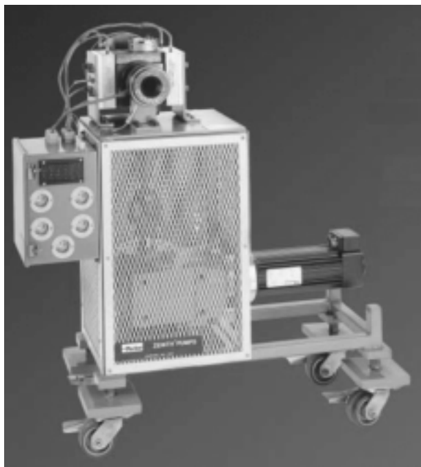
Figure 3. Melt pump assembly with motor drive. (Courtesy of Zenith Pumps)
