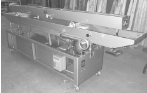
Figure 6. 10-foot free extrusion cooling tank. (Courtesy of RDN Manufacturing)
