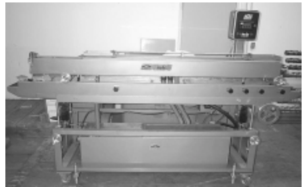
Figure 7. Vacuum sizing and cooling tank. (Courtesy of RDN Manufacturing)
