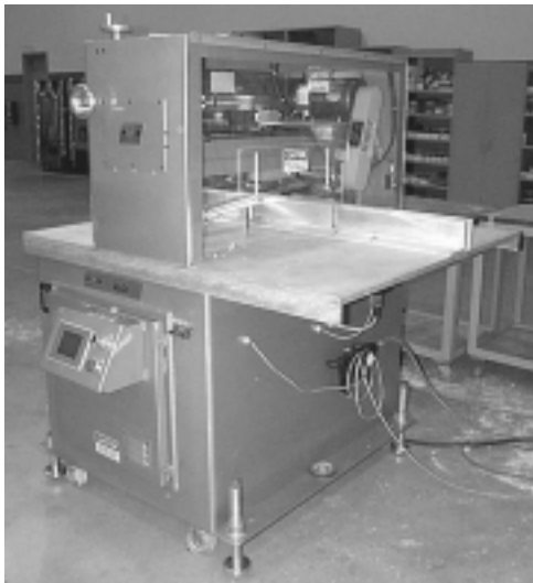
Figure 12. Top-cut traveling cut-off saw. (Courtesy of RDN Manufacturing)
